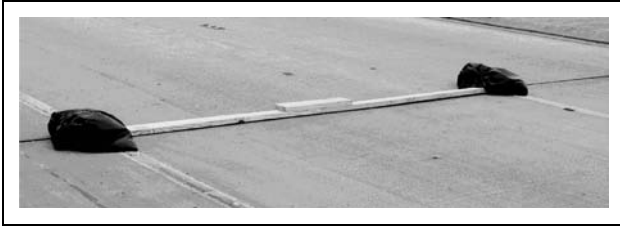
Figure 6. Changing the road surface condition by using a wooden bump.
