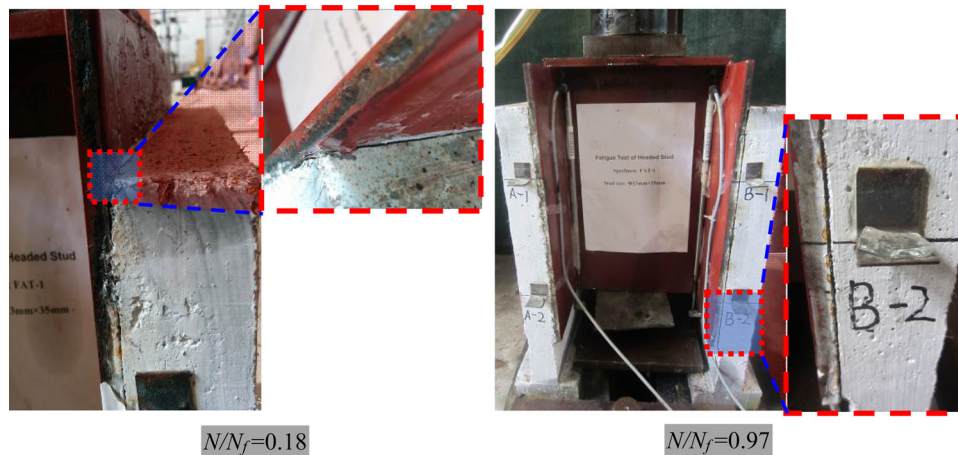
Fig. 19. Slip cracks observed at Side B of Specimen FAT-1
