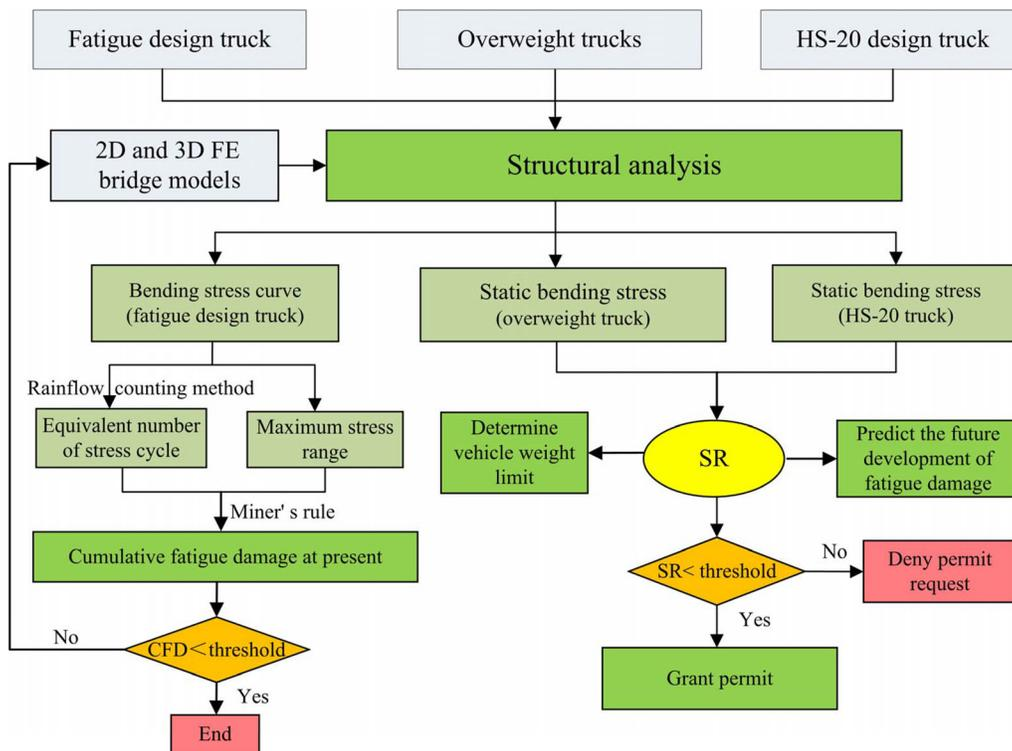
**Fig. 5.** Flowchart for determining vehicle weight limit and making permit decision.
