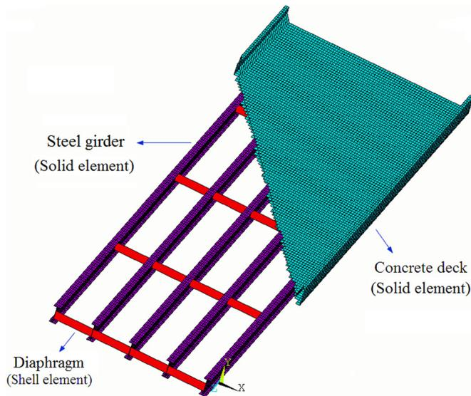
Fig. 3. 3D FE model of the bridge considered.
