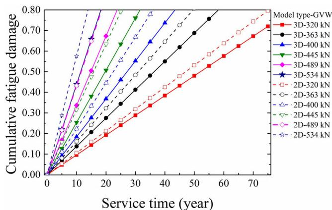
**Fig. 6.** CFD due to trucks with different GVWs with an assumed ADTT of 2,000.
