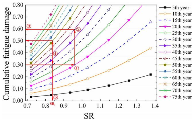
**Fig. 8.** Development of fatigue damage under different threshold values of SR.
