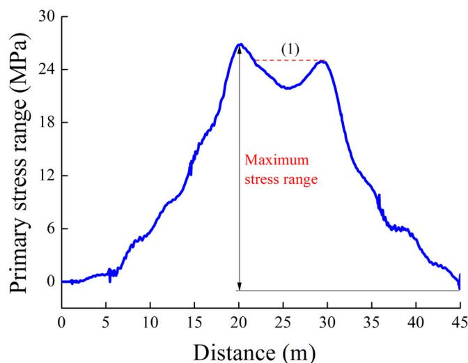
Fig. 4. Static stress history of the design fatigue truck.
