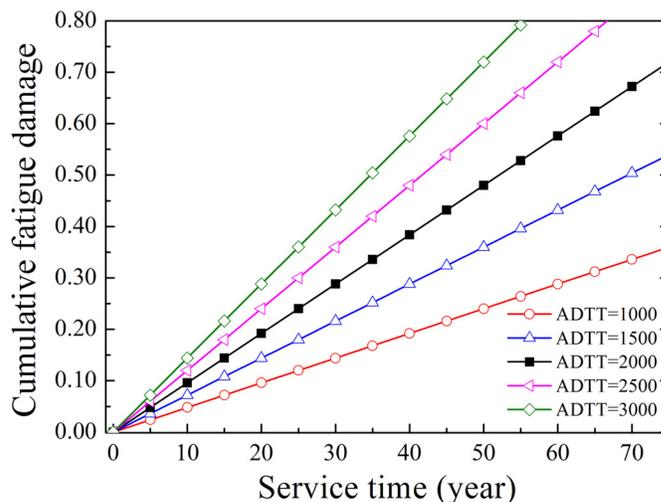
**Fig. 7.** CFD due to various ADTTs.
