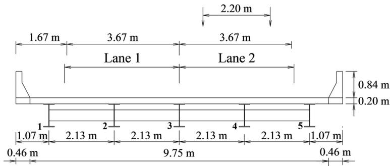
Fig. 2. Cross section of the bridge considered.
