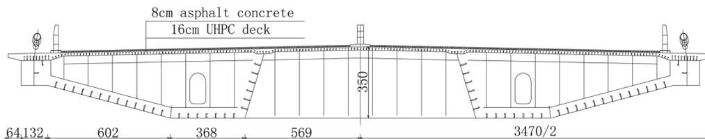
**Fig. 2.** Schematic of cross section of the main girder (unit: cm)
