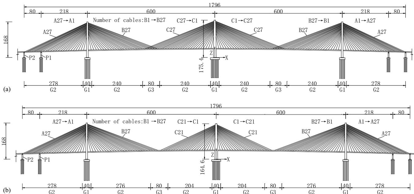
**Fig. 1.** Elevation layout of the bridge (unit: m); G1-G3 are girder section numbers, with section properties summarized in Table 1: (a) a conventional cable-stayed bridge with overlapping stay cables and (b) a proposed new cable-stayed bridge system
