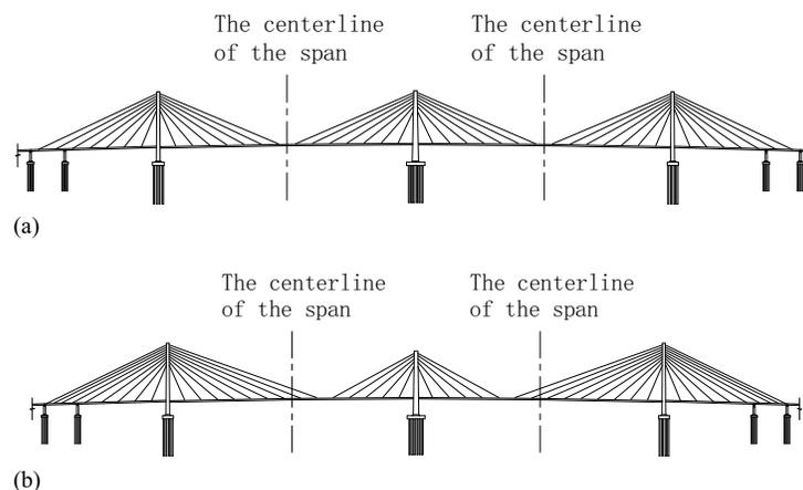
**Fig. 6.** Schematic diagram of cable-stayed bridge with size fans: (a) cable-stayed bridge with three equal-size fans (conventional system) and (b) cable-stayed bridge with two pairs of flanking tower cables crossing the midspan
