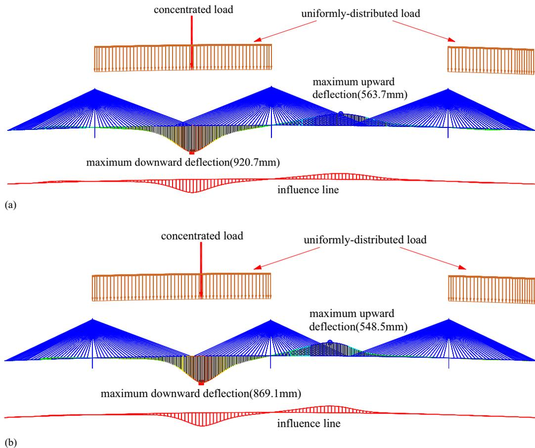
**Fig. 4.** The most adverse deformation of two different bridge systems: (a) a bridge with overlapping stay cables and (b) a bridge with unequal-size fans
