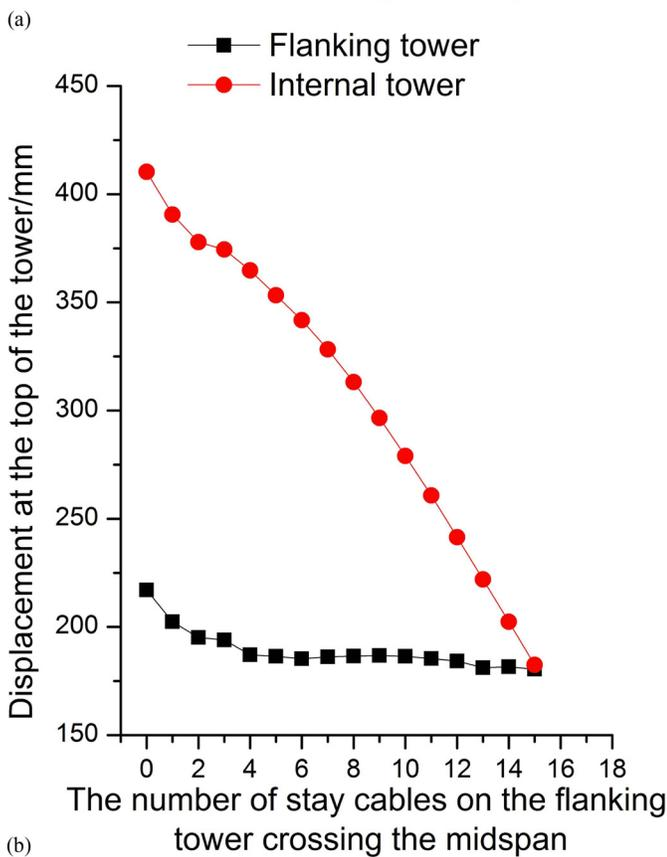
**Fig. 7.** Displacement of the proposed bridge system under the action of most unfavorable live load: (a) deflection of the main girder and (b) variation of the deflection at the top of the tower
