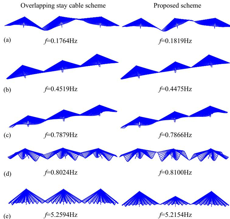
**Fig. 5.** Comparison of parts of vibration modes of two schemes: (a) 1st-mode shape, fundamental mode; (b) 9th-mode shape, lateral symmetric bending of the main girder; (c) 19th-mode shape, torsion of the main girder; (d) the 20th-mode shape, longitudinal floating of the main girder; and (e) 77th-mode shape, vertical symmetric bending of the main girder
