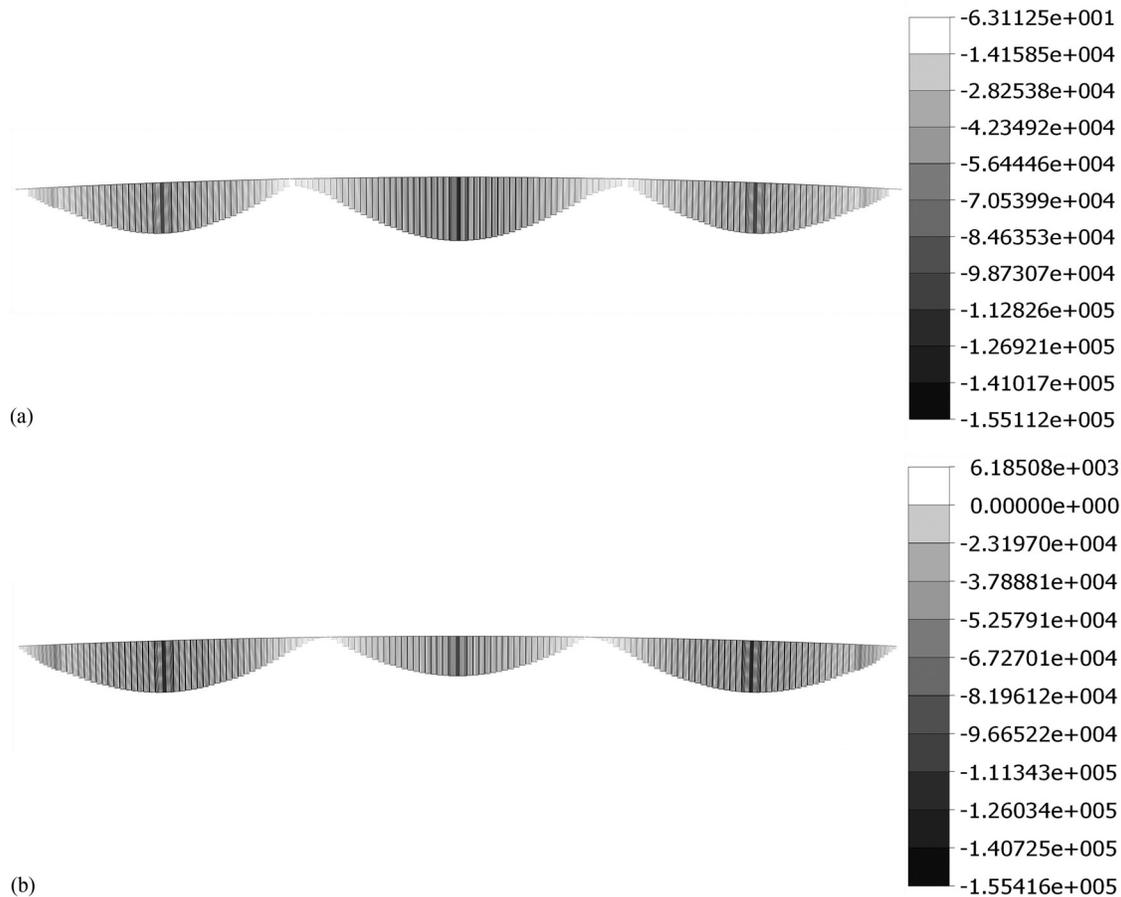
**Fig. 3.** Comparison of the axial force of the two different bridge systems under the dead load (unit: kN): (a) overlapping stay cables scheme and (b) proposed scheme
