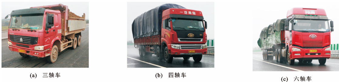
图9 现场试验车辆 Fig. 9 Vehicle in Field Test
