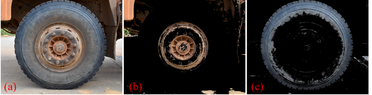
Fig. 6. Coarse segmentation using clustering algorithm: (a) original tire image; (b) rim edge segmentation; (c) tire edge segmentation.
