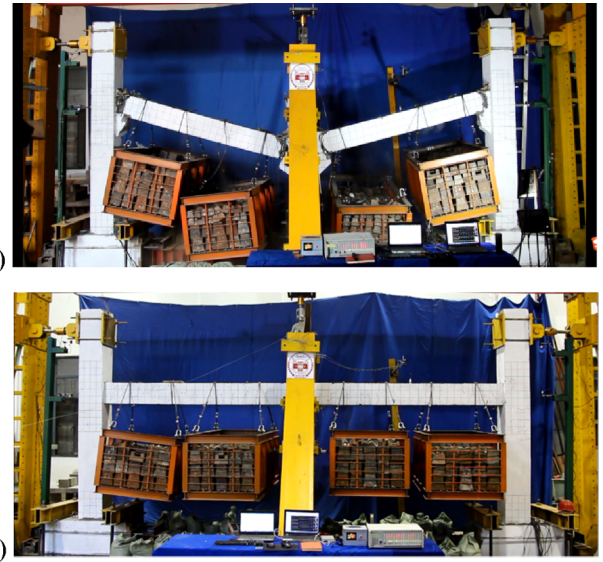
Fig. 5. Failure mode of specimens at the end of the 4th load step: (a) PC specimen; (b) RC specimen.
